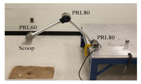
Figure 3.1: A robotic arm for sample retrieval
