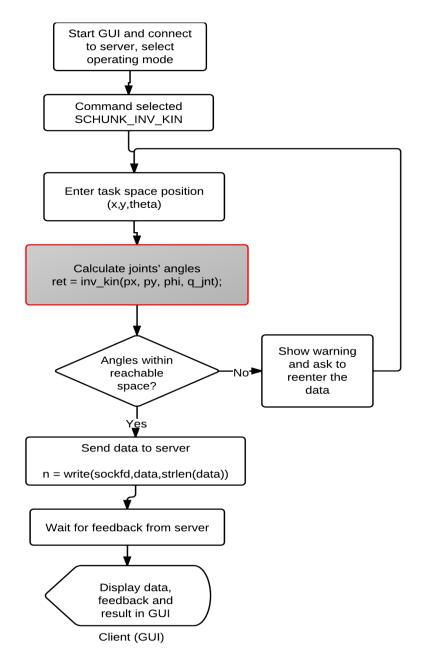
Figure 5.13: Process flow for task space control
