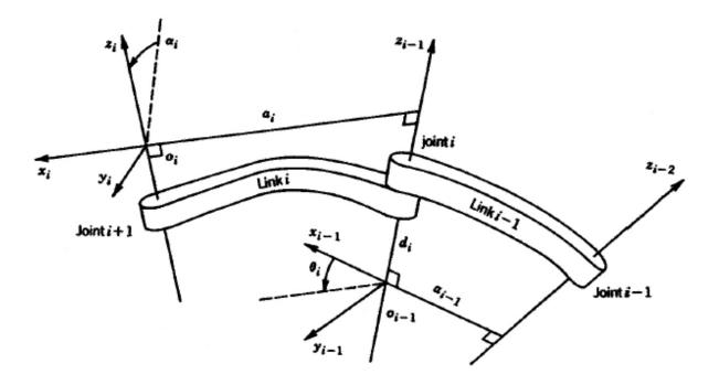
Figure 3.5: Frame assignment for the DH convention [24]
