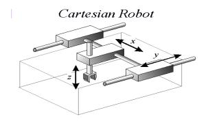
Figure A.3: Cartesian Robot<sup>3</sup>
