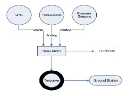
Figure 2.6: CanSat data flow block diagram [4]
