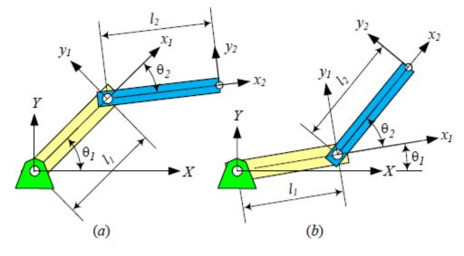
Figure 3.7: a) elbow-up, b) elbow-down configuration [11]
