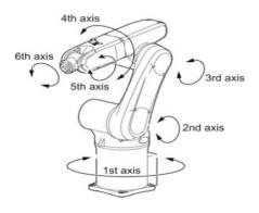
Figure A.5: Articulated Robot<sup>5</sup>
