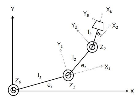
Figure 3.6: Model of robotic mast
