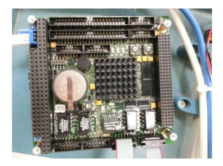
Figure 3.2: Embedded computer (PC/104)
