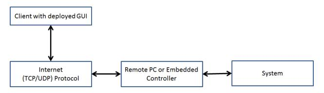
Figure 1.2: Block diagram of remotely controlled system
