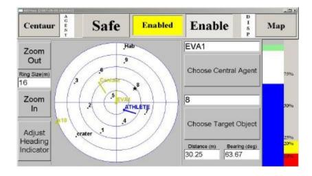
Figure 2.1: AIDMap GUI: Display of robots and known locations [10]
