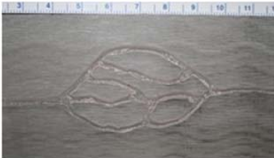
Figure 3-1: Rexolite® multichannel blood vessel phantom.
