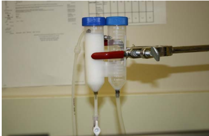
Figure 3-4: A photograph shows the head and over flow containers that were used to convert the pulsatile flow to steady flow, as well as the manual valve tap that was used to control the fluid flow.
