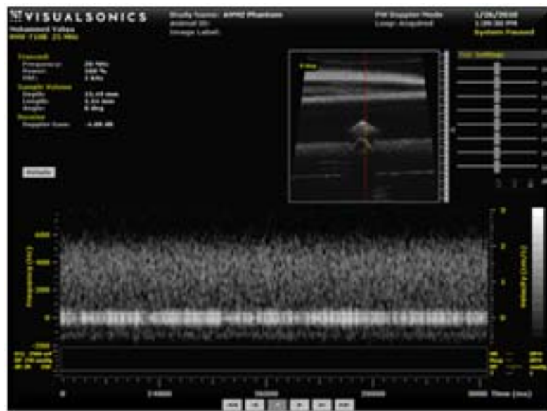
Figure 3-7: Video Display of Vevo770® scanner for the Continues Velocity on the Blood Vessel Phantom.
