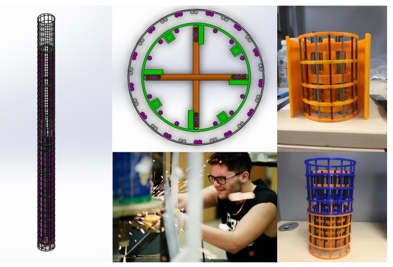
Figures 2-6: Pictures of thermal caisson CAD model, 3D printed models, and me assisting in the setup of a bench-scale test
