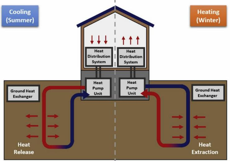
Figure 1: Diagram of a basic GSHP system [1]
