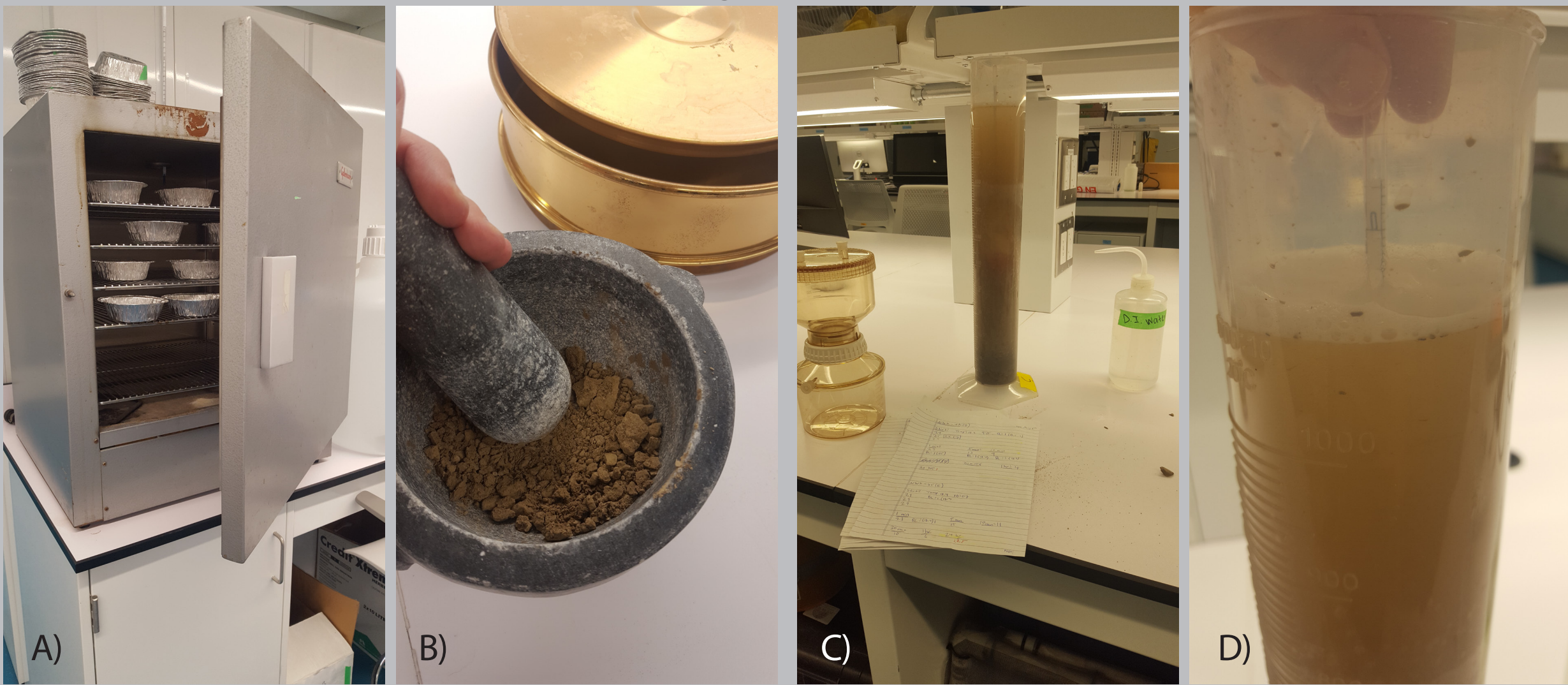
Figure 1 Hydrometer Texture Analysis Procedures. A) Oven Drying Soil Samples, B) Grinding Soil, C) Sediment in Suspension, D) Measuring Solution Density
