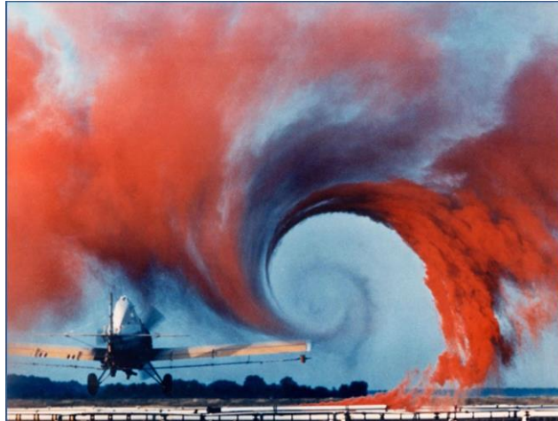
Figure 1.2: Trailing wingtip vortex created by an aircraft [2].
