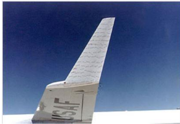
Figure 1.1: Winglet on KC-135 test aircraft, with tufts displaying flow of air over winglet surface [1].
