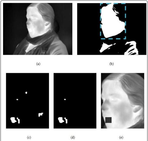
**Figure 1 Visual representation of the infrared thermal switch video processing algorithm**. (a) Input grayscale thermal video frame, (b) Result of face localization, (c) Result of intensity analysis (warm area mask), (d) Intersection of warm area mask and motion mask, (e) Open mouth detected and marked on the video. Note that for ease of visualization, images (c)-(e) only show the smaller region demarcated by the dashed box in (b).
