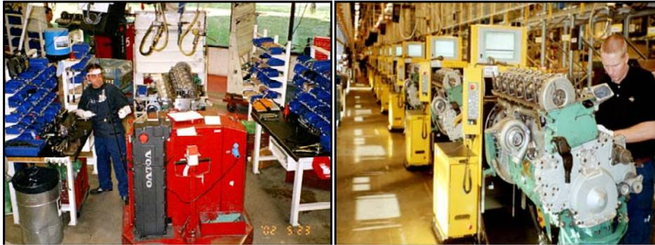
**Figure 2: Schematic and picture for both long-cycle parallel flow assembly system (Left) and serial flow line assembly system (Right)**
