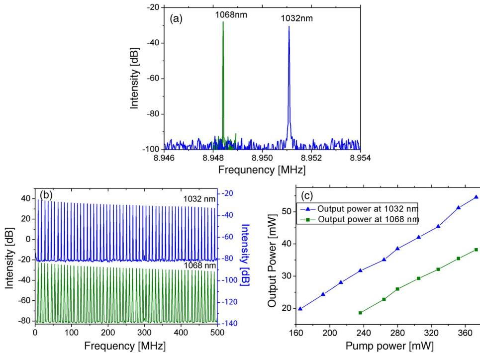
Fig. 5. RF spectrum (a) around the fundamental and (b) harmonic repetition rates at 1032 nm and 1068 nm. (c) Output power of the mode-locked fiber laser with respect to the pump power at 1032 nm and 1068 nm.
