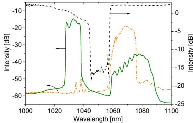
Fig. 3. Transmission spectrum of chirped FBG (dash), output spectrum of the mode-locked fiber laser at 1032 nm (solid) and 1068 nm (dash dot).
