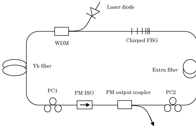
Fig. 1. Schematic diagram of the mode-locked fiber laser.
