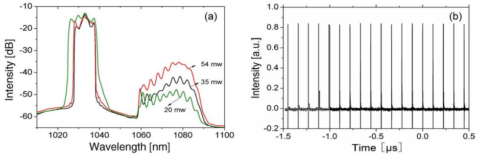
Fig. 2. (a) 1032-nm output spectra of the mode-locked fiber laser at different output power (20 mW, 35 mW, 55 mW). (b) Output pulse trains of 1032-nm mode-locked laser.
