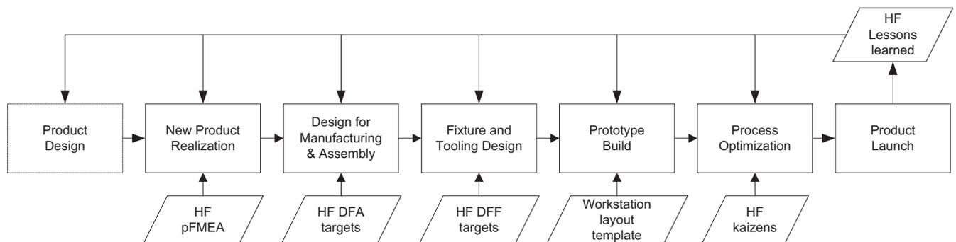
**FIGURE 2** Integration of tools adapted for HF in the design process.
