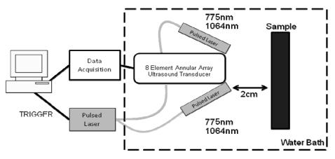
Figure 1. Schematic representation of the optoacoustic imaging system
