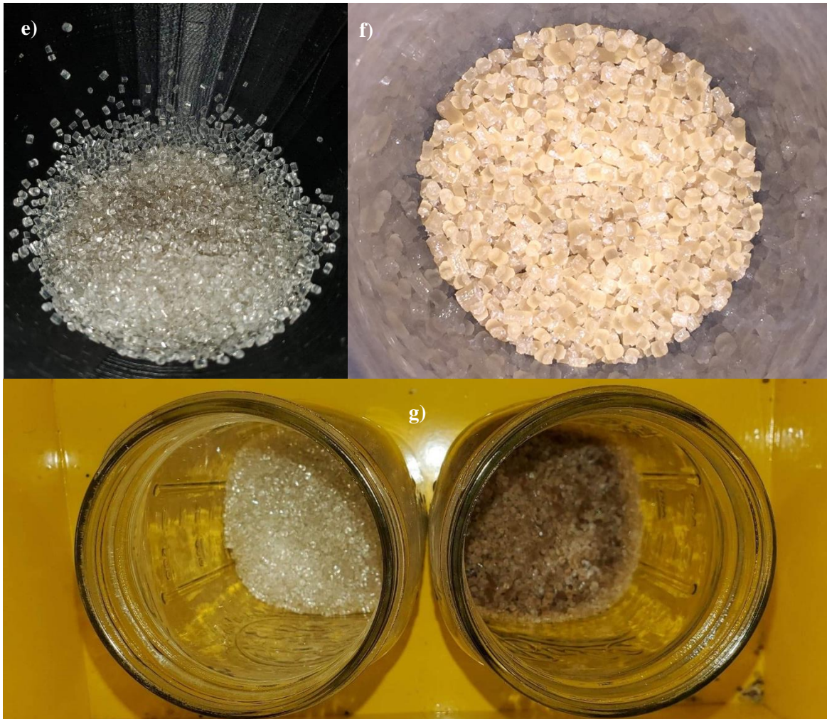
Figure 28. Preparation of: (e) PLA; (f) 3% pyro-RFG-PLA pellets; and (g) in dehydrator.
