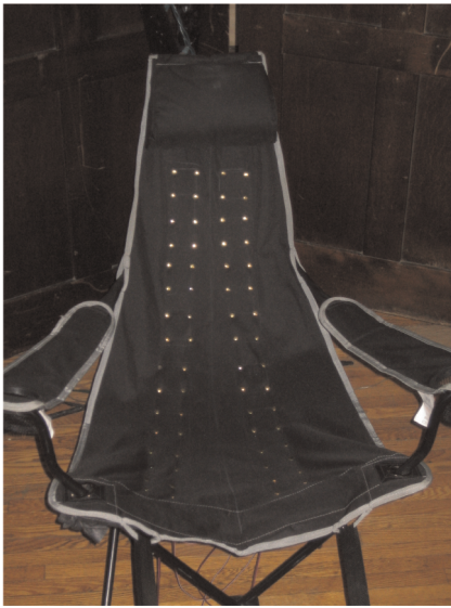
Fig. 8. The current MHC prototype uses 16 voice coils in a 2 \times 8 configuration. Voice coils are attached to the back of the chair, with four upholstery pins securing each in place.
