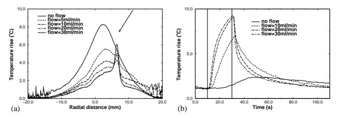
Figure 1: Steady state (a) and transient (b) temperature profiles measured by a scanned thermocouple. Arrow indicates location at which transient temperature profile was measured in (b). Vertical bars indicate the pulse on and off times. Note the distinct peak in (a) and the transient response at that location in (b).
