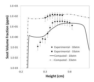
Figure 5: CoFlame computed centreline soot volume fraction profile compared with experimental data for ethane-air diffusion flames at 10 and 33 atm with experimental air flow rate. [9, 10]
