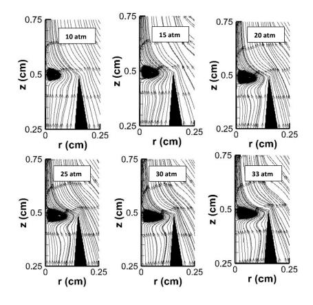
Figure 3: Computed flow streamlines with the CoFlame code near fuel tube tip for an ethane-air diffusion flame at 10 (top-left), 15 (top-middle), 20 (top-right), 25 (bottom-left), 30 (bottom-middle), and 33 (bottom-right) atm.
