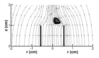
Figure 1: Computed flow streamlines for the CoFlame code near the fuel tube exit plane for an atmospheric methane-air diffusion flame on the left side, and an atmospheric propane-air flame on the right side.
