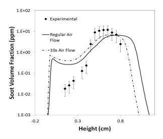
Figure 4: CoFlame computed centreline soot volume fraction profile compared with experimental data for ethane-air diffusion flames at 5 atm with experimental air flow rate and ten times the experimental flow rate. [9, 10]
