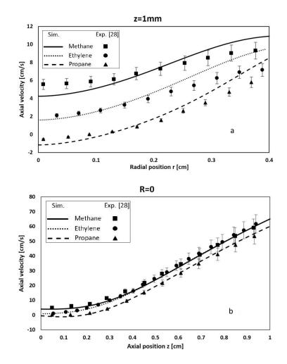
Figure 2: Comparison of the numerical and the experimental results of the radial (a: at z = 1 mm) and axial (b: at R = 0) profiles of the axial velocity for methane, ethylene, and propane flames
