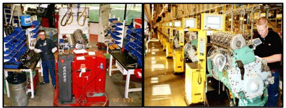
Figure 1: OLD system dock workstation (left) & NEW line system (right)
