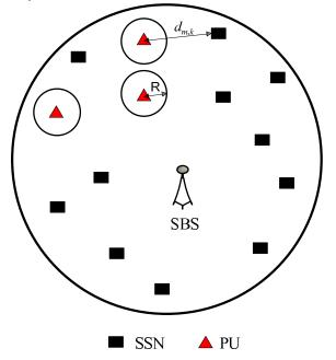
As shown in Figure 1, there is a PU protection area, wherein the strengths of the SSN signals must be constrained. We define as R, the radius of the protected circular area for each individual PU. Given a distance,  $d_{m,k}$ , between the kth SSN transmitter and the mth PU and the radius,  $R_m$ , of the protected circular area of the mth PU, the channel from the source to the mth PU in the kth SSN frequency band is given as:
