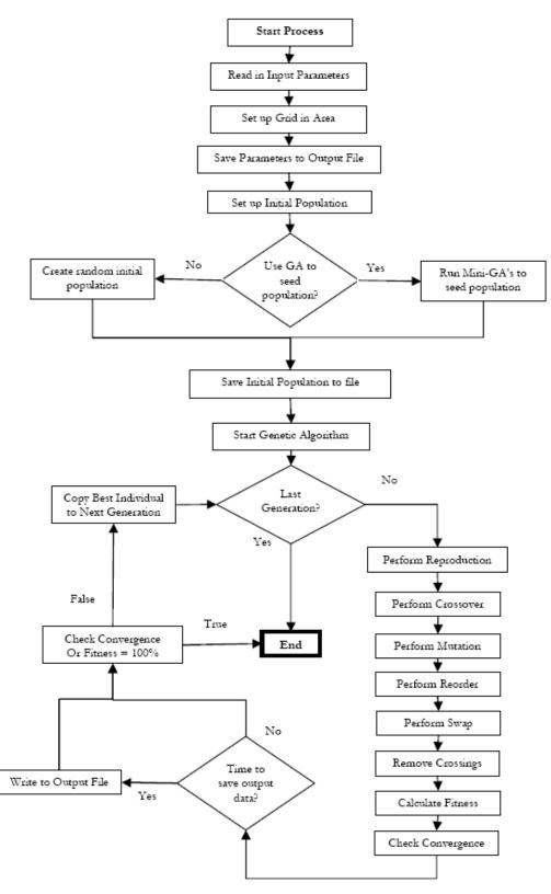
Figure 3. Flowchart of genetic algorithm (GA) based path planner.
