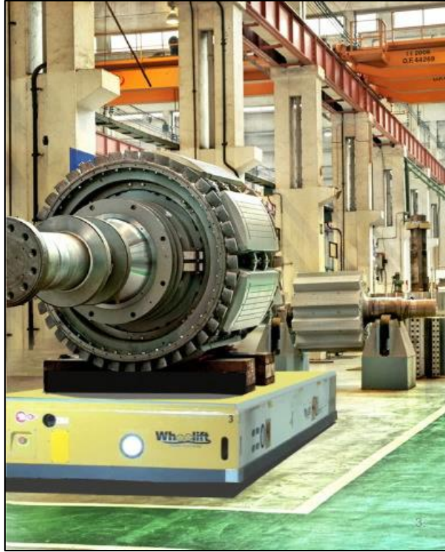
Figure 5. An RGV transporting equipment in an industrial plant. [R.3]
