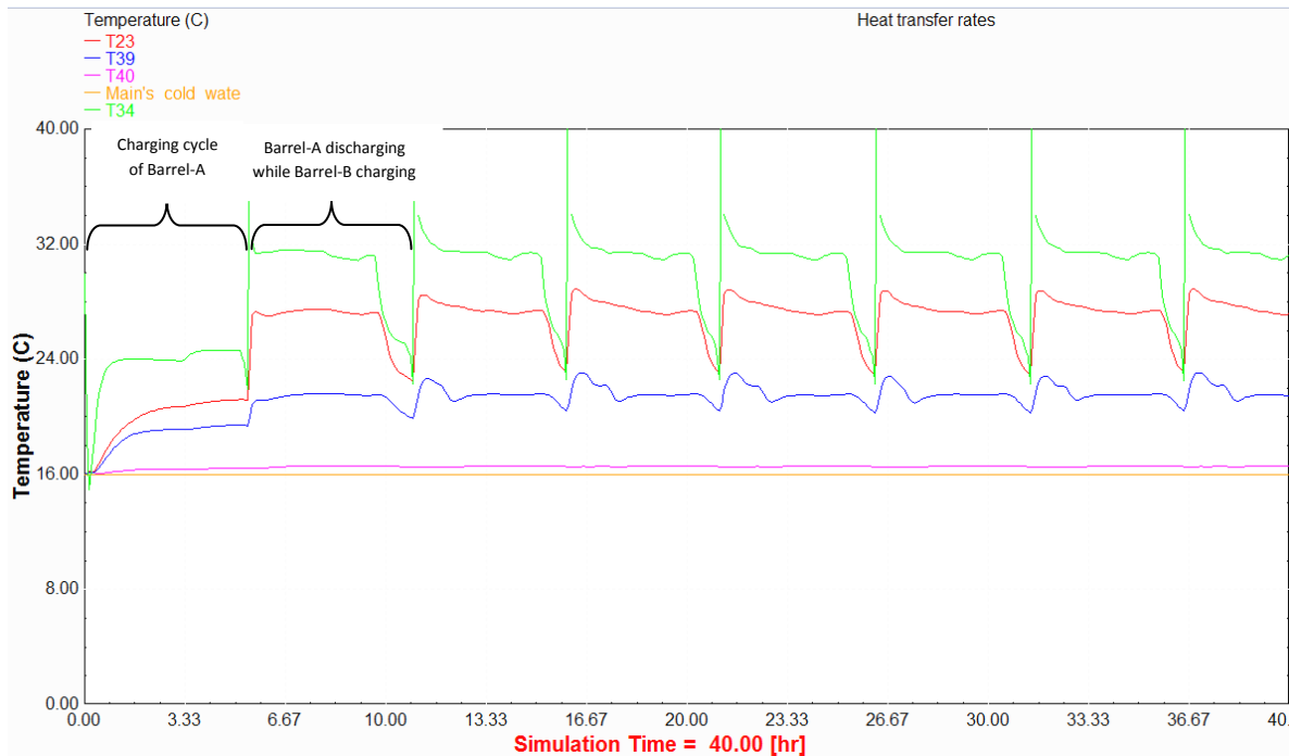
Figure 6.9 Simulation result for temperature vs. time at different points of the tri-generation system
