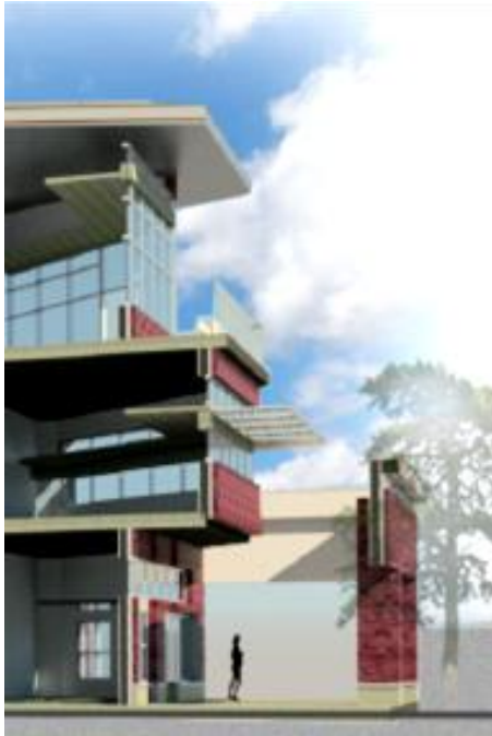
Figure 43 - Final design: metal grille shading devices on south facade with light shelves extending inside the space
