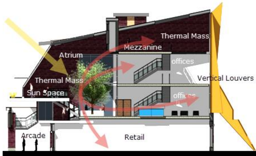
Figure 42 - Passive Heating Strategies: Section through central atrium: a) Direct Heating Gain, b) Isolated Solar Gain, c) Thermal Mass, and d) Convective Heating from atrium to interior spaces.
