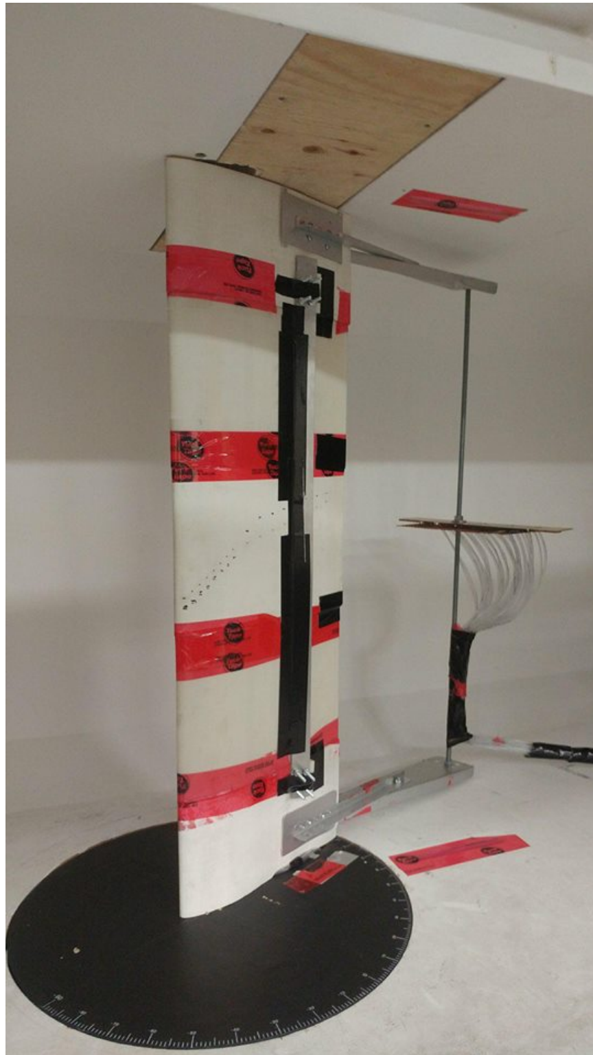
Figure 2.8: Wind tunnel model fully assembled and mounted in the Ryerson Large Wind Tunnel.
