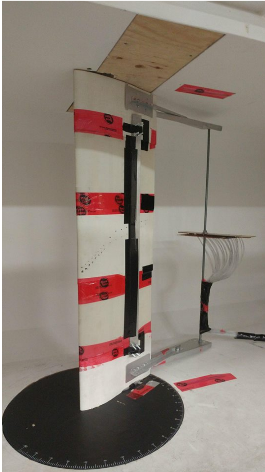
Figure 2.1: Wind tunnel model fully assembled and mounted in the Ryerson Large Wind Tunnel.
