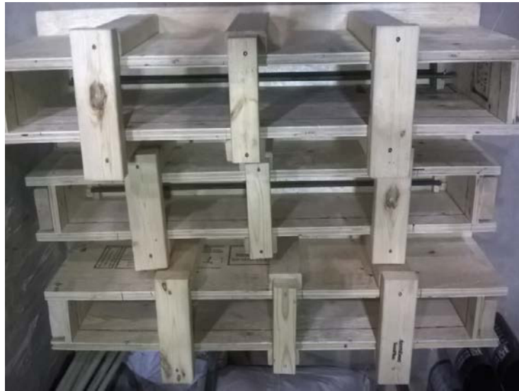
Figure 3.11(a) - Mould or formwork showing reinforcement casing
