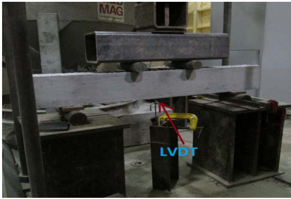
Figure 3.14 -Shear beam experimental set-up and instrumentation
