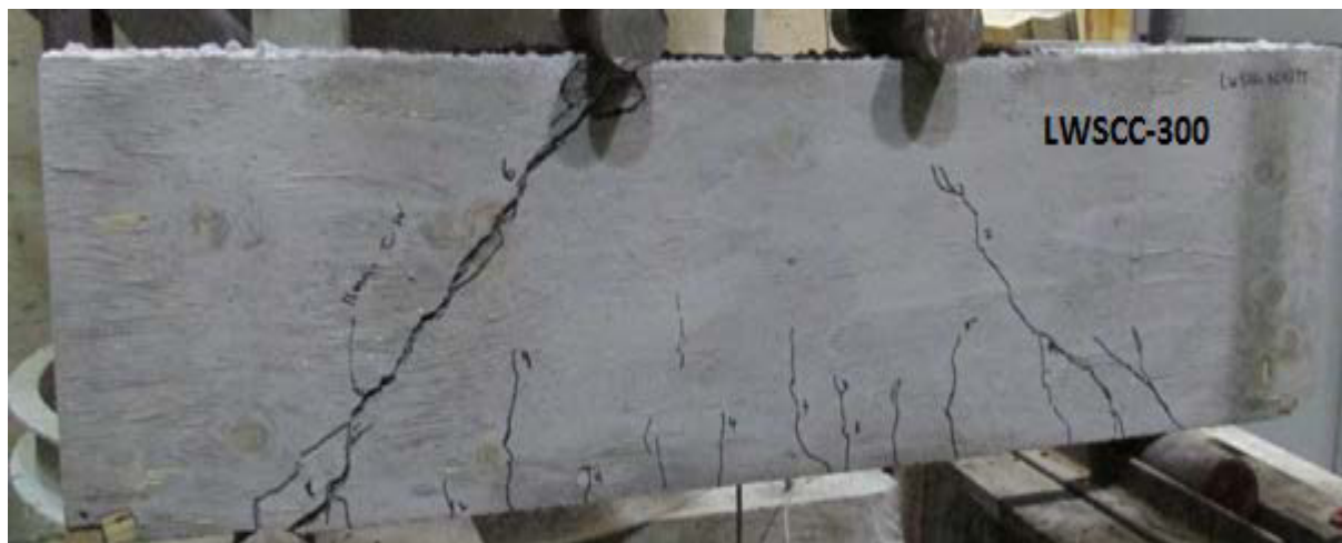
Figure 4.2(a) - Failure modes tested shear LWSCC beams without shear reinforcement
