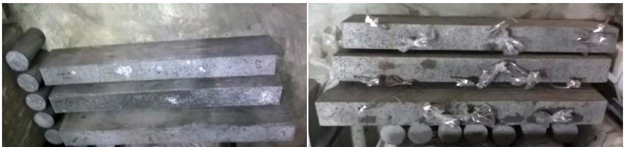
Figure 3.13- Air curing of beams and control specimens
