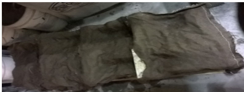
Figure 3.12- Moist curing of beams and control specimens
