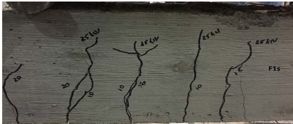
Figure 4.10(a) - Crack pattern and failure mode of singly reinforced F1s flexural beam
