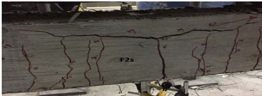
Figure 4.10(b) - Crack pattern and failure mode of singly reinforced F2s flexural beam
