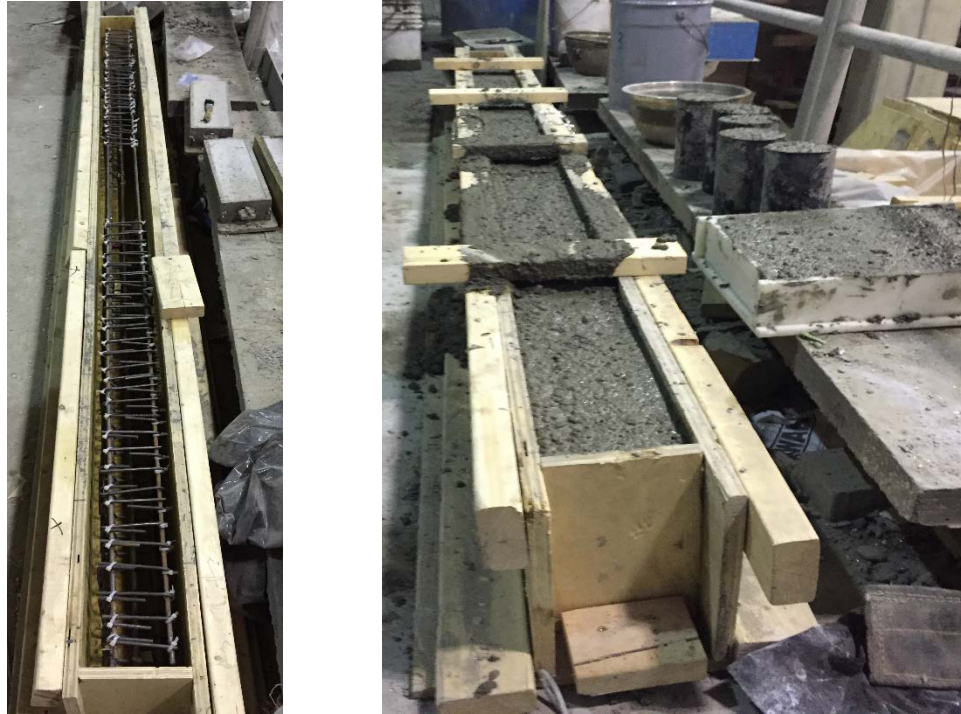
Figure 3.11 (c) - Beam formwork and casted beam
