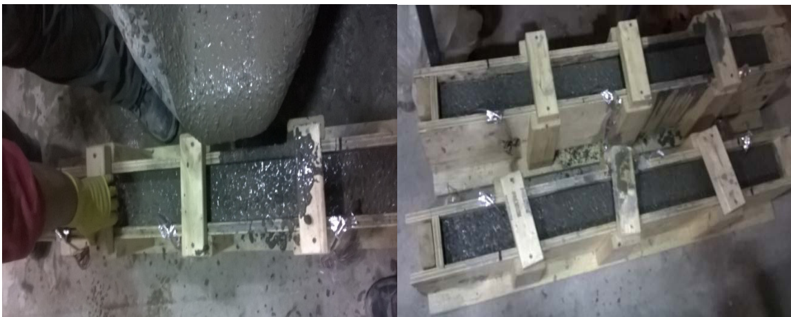
Figure 3.11(b) - Beam casting showing concrete pouring and casted beams
