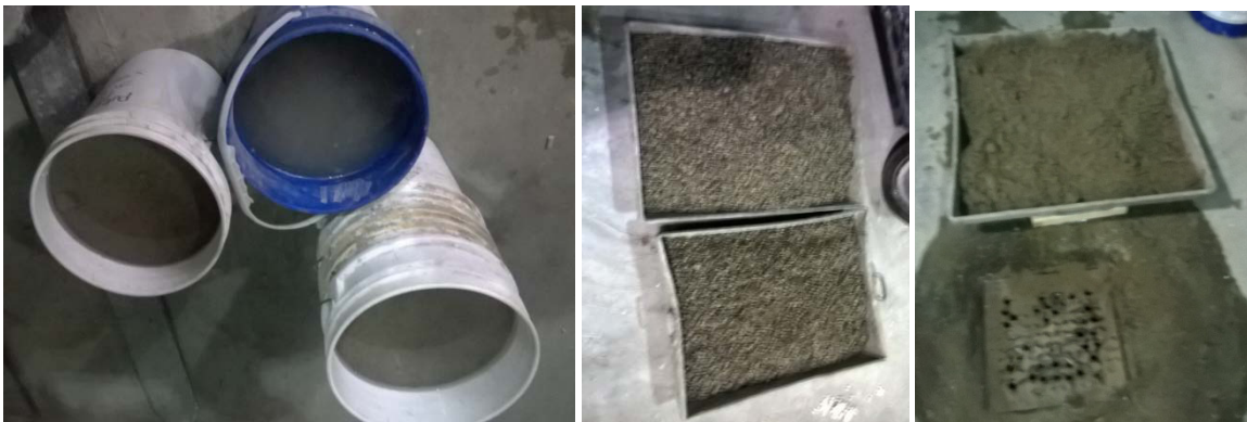
Figure 3.8-Slag aggregates -72 hours pre-soaking
