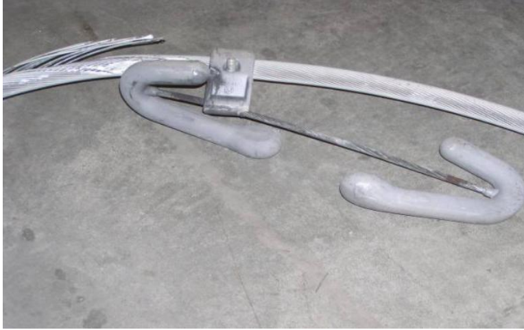
Figure 1.2: Broken conductor strand and slippage of the messenger wire of the Stockbridge damper [6].
