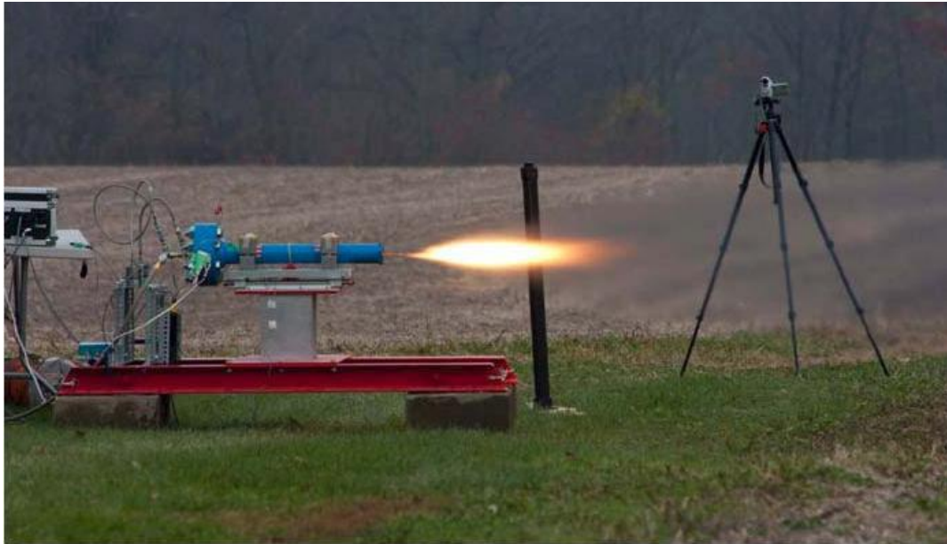
Fig. 3.8: Photo of Ryerson University labscale hybrid rocket engine (LDPE / GOx) being fired at Continuum Aerospace test site [5]
