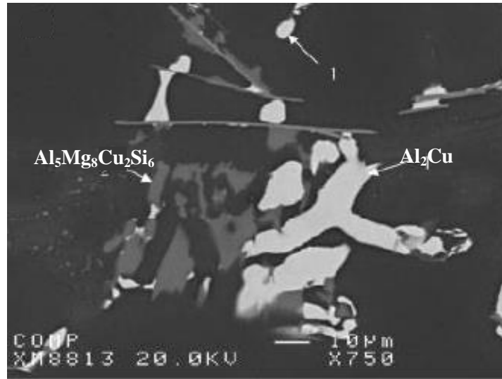
Figure 2.4: Backscattered electron image showing the morphology of blocky \text{Al}_2\text{Cu} in clusters with blocky \text{Al}_5\text{Mg}_8\text{Cu}_2\text{Si}_6 [21].
