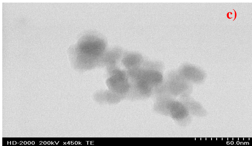
Fig 6.2 SEM and TEM micrographs of the laser irradiated PDMS coated aluminum sample surface and the nanoparticles aggregate respectively. (a) Surface featuring web like nanoparticles around the laser spot, (b, c) PDMS-Al /Al nanoparticles in the aggregate structure
