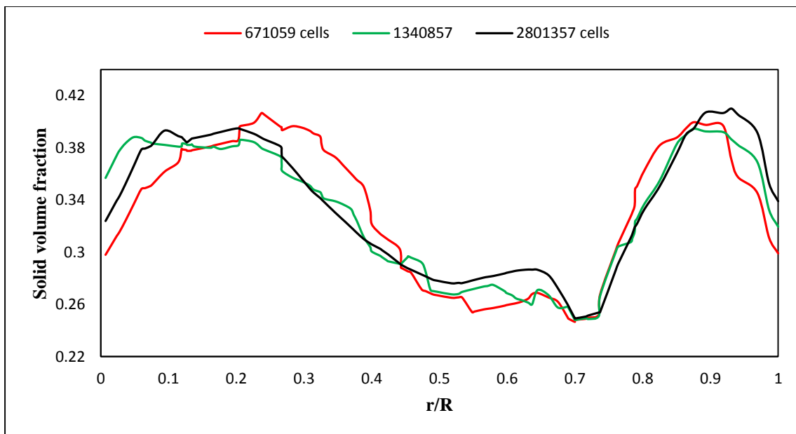
Figure (4.4-2). Grid independency: Solid concentration profiles at 1.5 cm below the Maxblend impeller ( N = 480 rpm, X = 30 wt%, d_p = 209 \mu\text{m} , C = T / 8 ).
