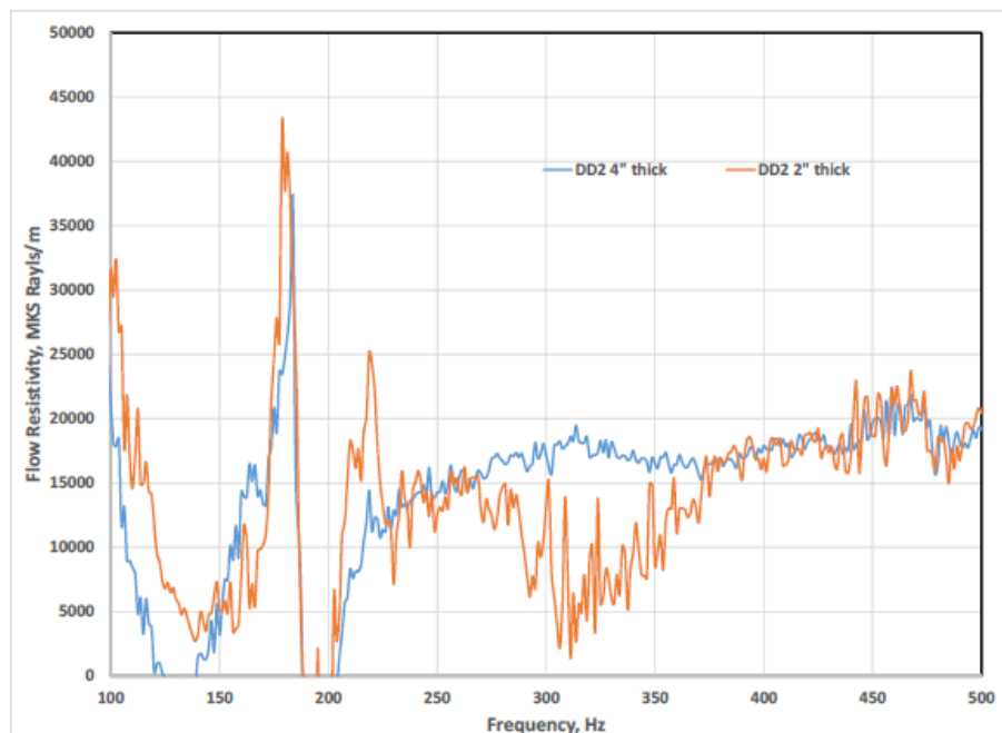
Figure 6.17- Three microphone method: Flow resistivity of DD2 4\" sample [39]
