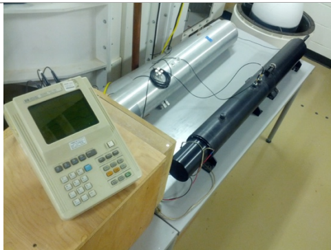
(a) Circular impedance tube and FFT Analyser
