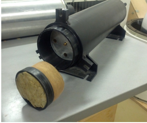
(a) Custom Ring Used to Fit Samples
