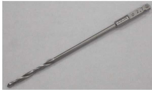
Figure 4-5: A stainless steel, 2.7mm diameter orthopaedic surgical drill bit used for experiments.
