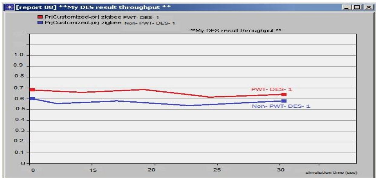
Figure 34: Throughput of Both scenarios in a network with 60% M2M devices vs. simulation time
