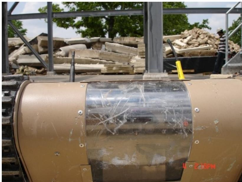
Figure 3.3 – Matilda robot with scratched and abraded armoured front visor. Damage caused by attempting to traverse rubble seen in background
