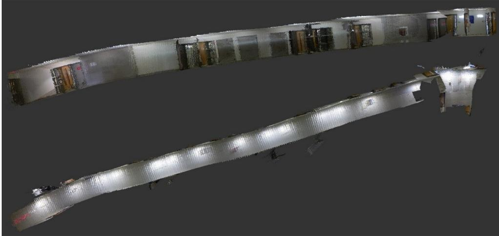
Figure 4.14 – Top and side view of model created by SURF + descriptor matching in Environment 2 (narrow hallway)
