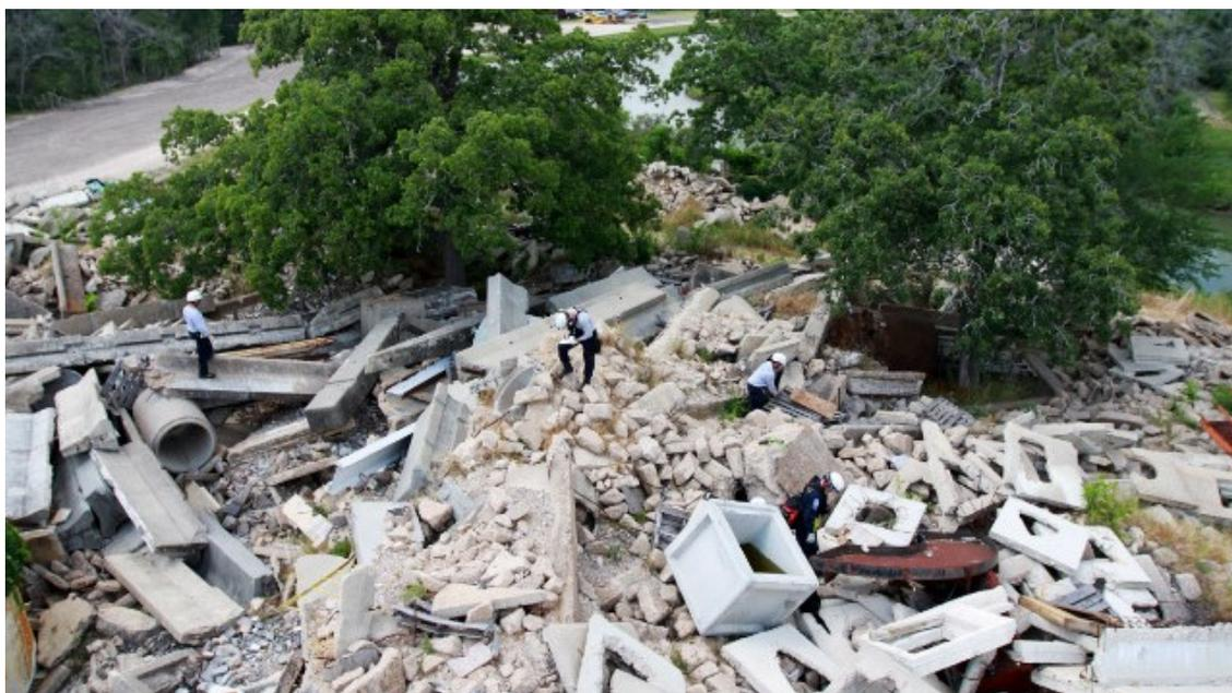
Figure 3.4 – Purpose built rubble pile for USAR training at “Disaster City”
