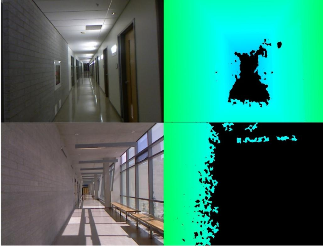
Figure 4.8 – The effect of ambient sunlight on Kinect depth data. black regions show where the Kinect failed to measure the depth
