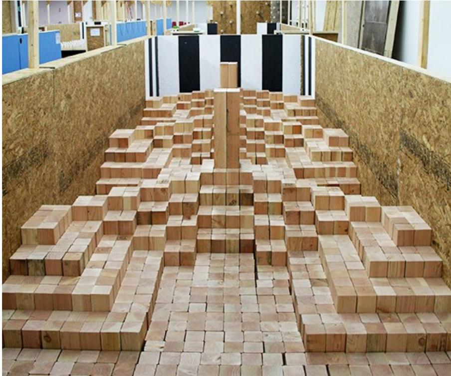
Figure 3.5 – An example of a robot test “step field” in one configuration of a NIST mobility test
