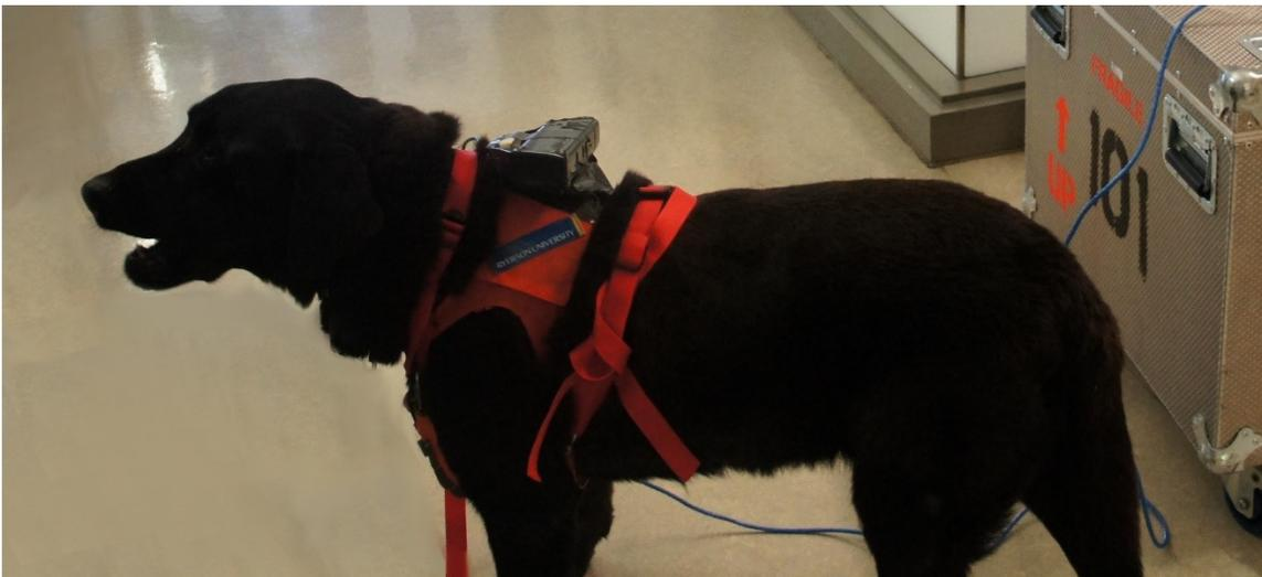
Figure 5.1 – RGB-D Sensor mounted on search dog Dare
