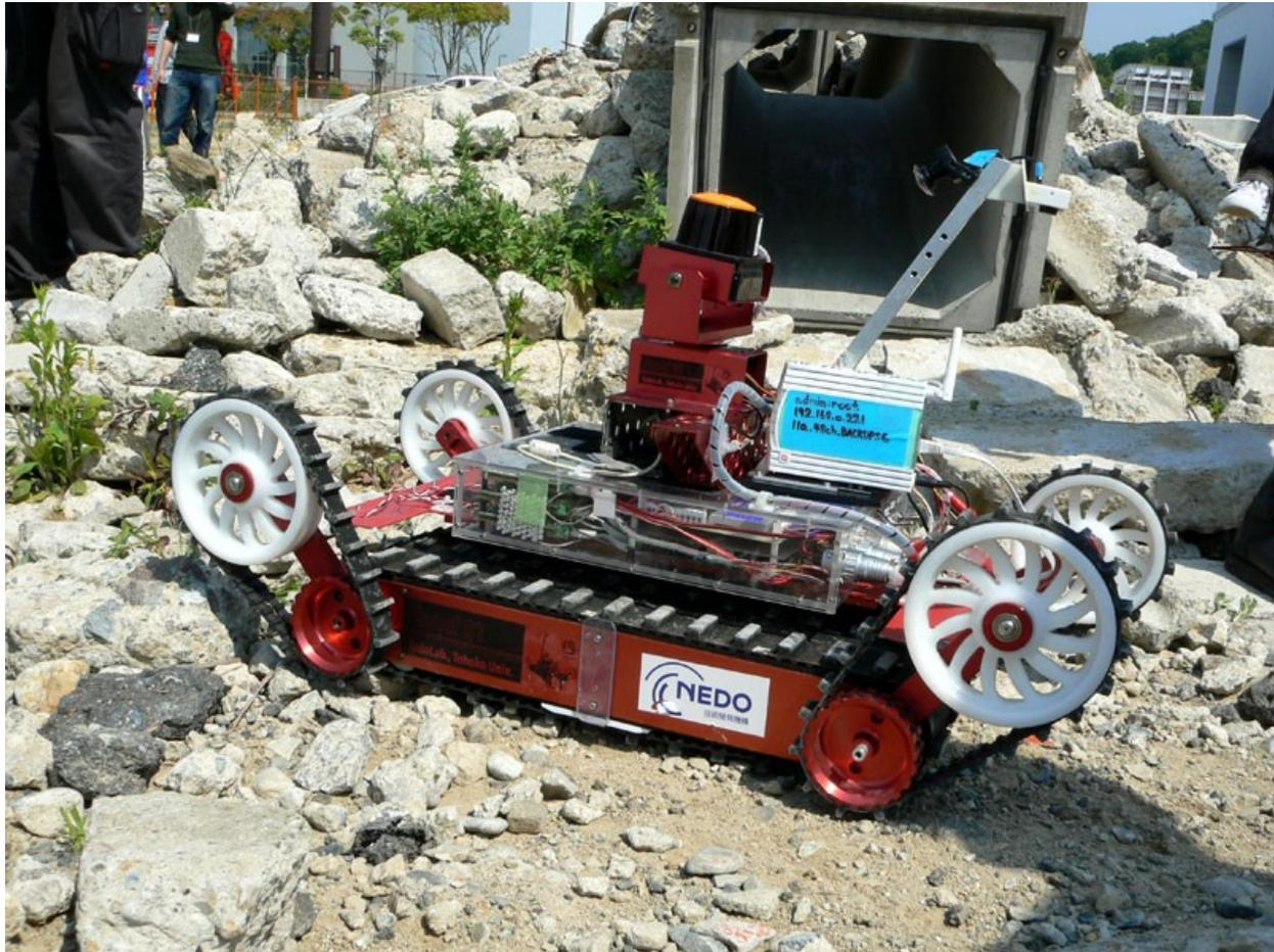
Figure 3.1 – Kenaf rescue robot with features including crawler enclosing its entire body and four sub-crawler arms that are each controlled independently [40, 41]
