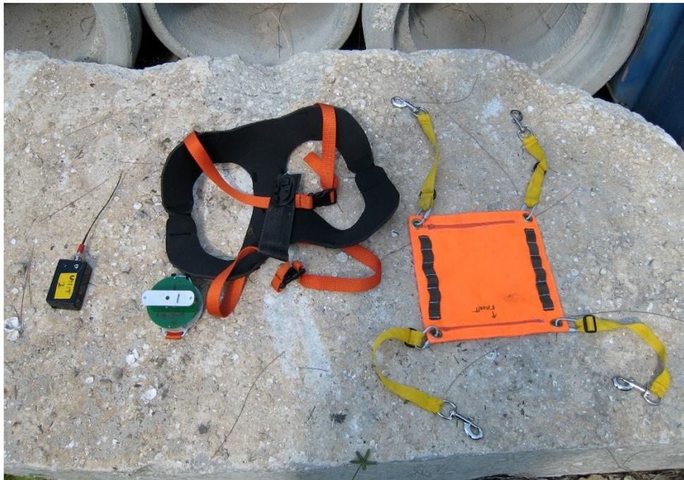
Figure 2.6 – CRDS detail. From left to right: Remote, CRDS, harness, underdog
