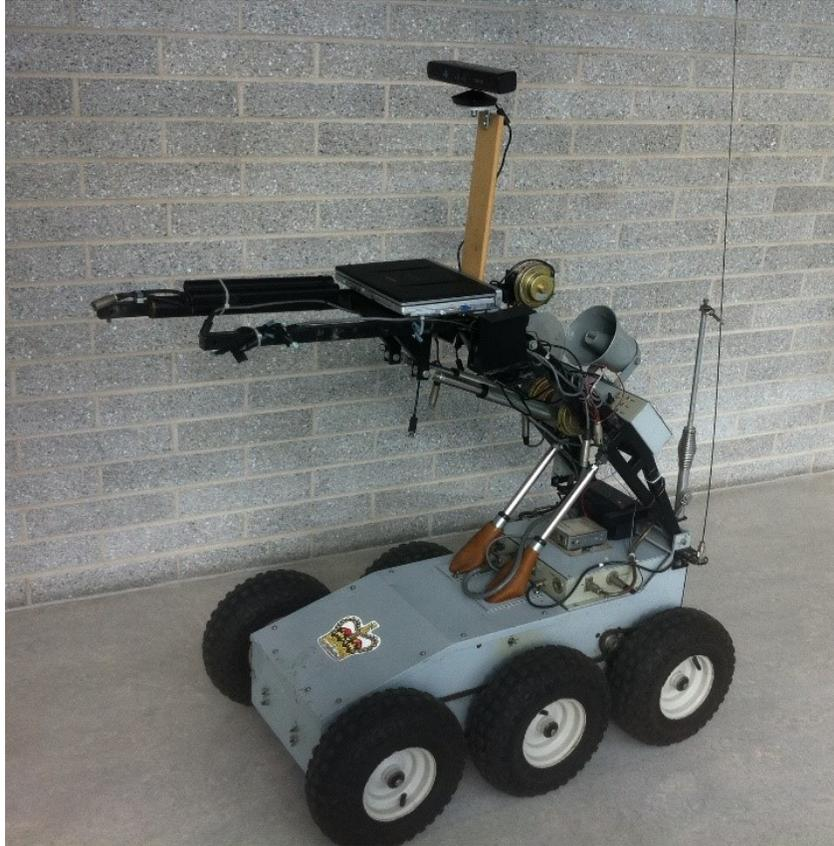
Figure 4.7 – Pedasco RMI-9WT Remote Mobile Investigator equipped with Kinect sensor
