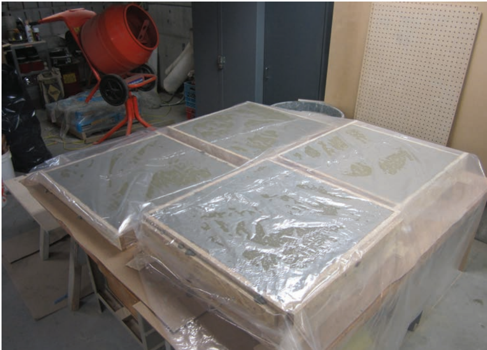
Figure 55: MV4 Concrete Panels Curing
