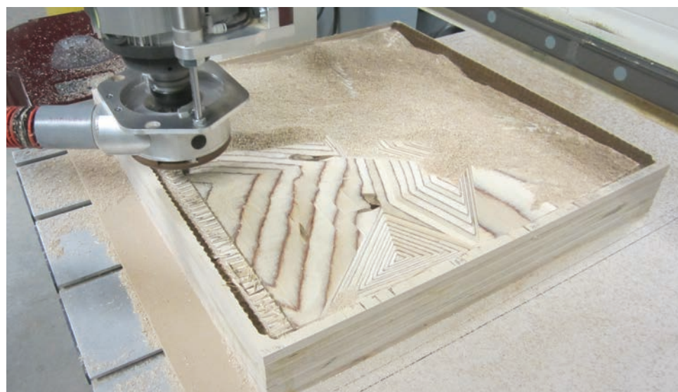
Figure 131: CNC Milling Concrete Form derived from Rhino Model
