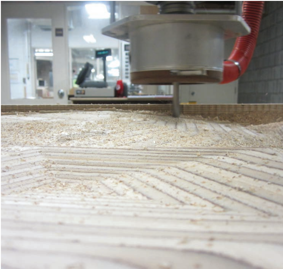
Figure 05: CNC Cutting Concrete Form
