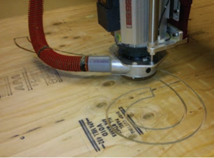
Figure 20: CNC Milling Formwork
