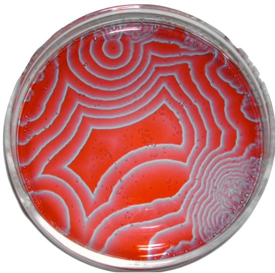
Figure 3.3. An active Belousov-Zhabotinsky reaction
