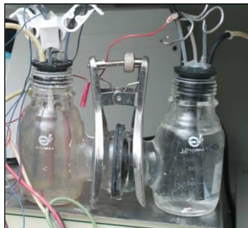
Fig. 2.1 a. Schematic of ethanol fed MEC b. Ethanol fed MEC with graphite electrodes, inoculated with anaerobic digested and waste activated sludge, and run at Arizona State University.
