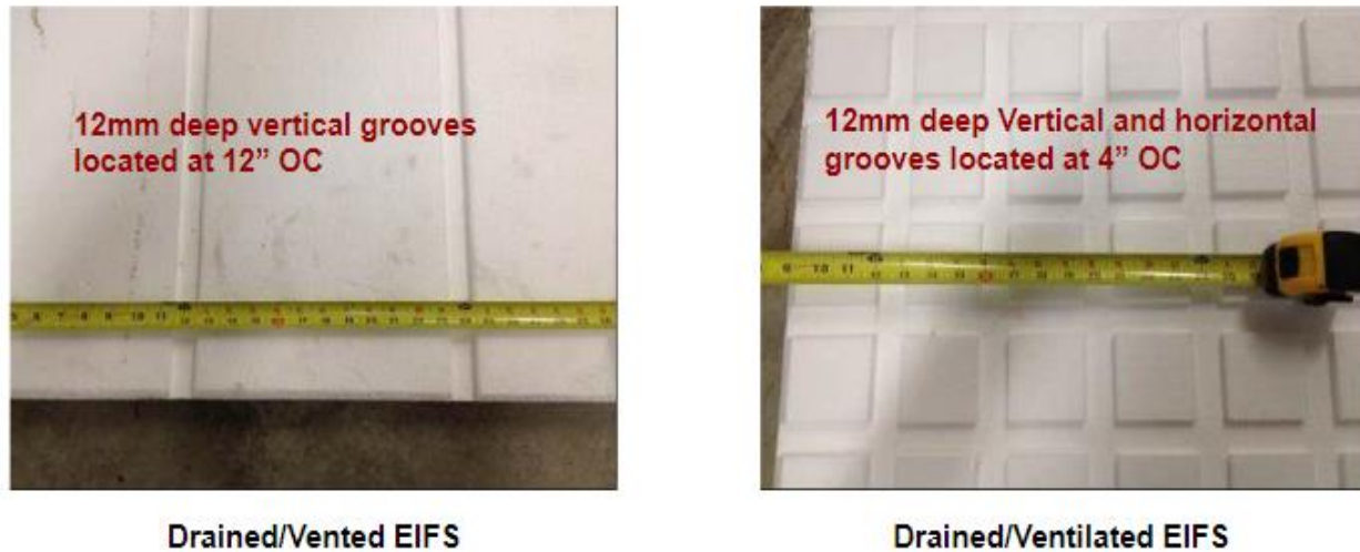
Figure 3. Vented Vs. Ventilated EIFS. (Smegal, 2017)
