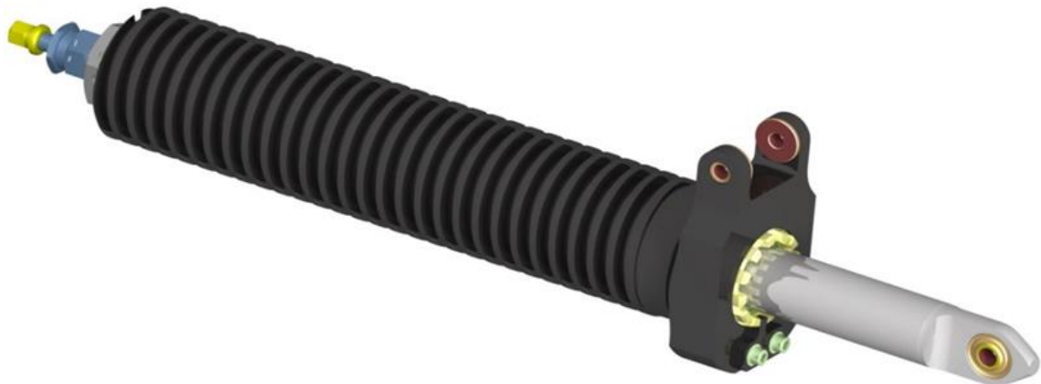
Figure 4.12: The HDWS Shock Strut sub-assembly, CATIA® V5 rendering
