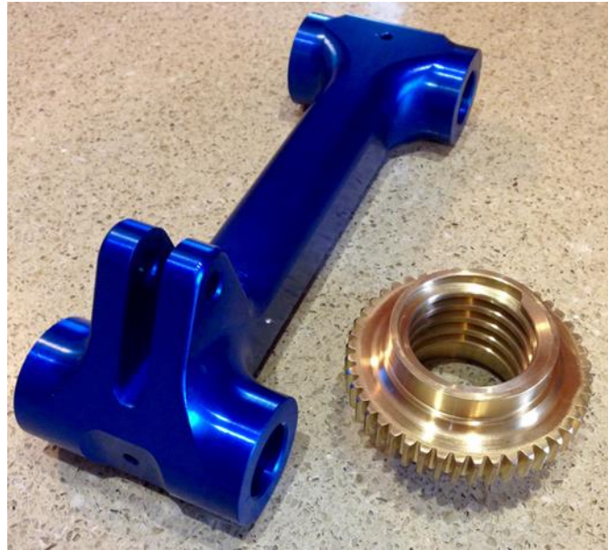
Figure 4.31: Trailing arm pictured after undergoing blue anodizing
