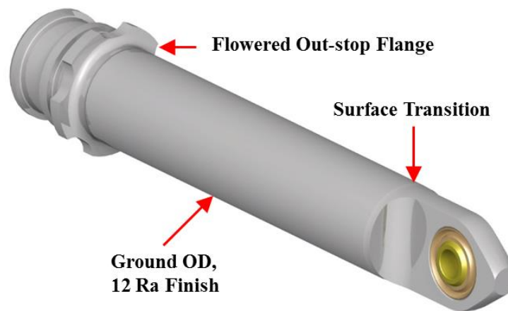
Figure 5.19: 3D view of the piston, spherical bearing installed, key features labeled
