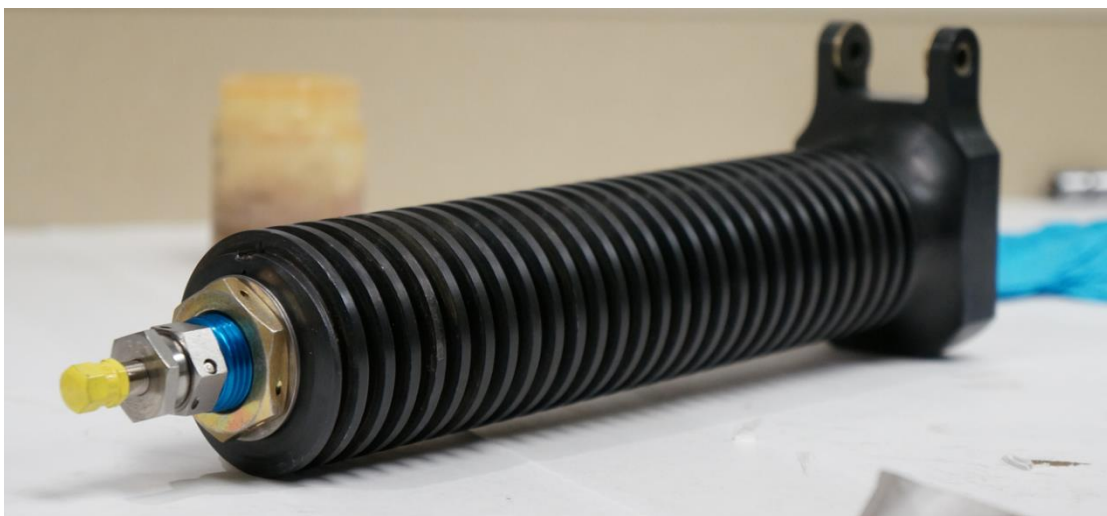
Figure 4.32: A shock strut outer cylinder shown with black oxide surface treatment
