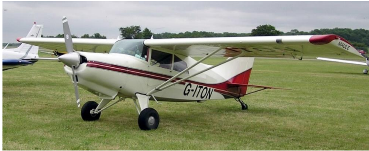
Figure 2.6: Tail wheel configuration landing gear on a STOL Maule MX-7-235 Super Rocket
