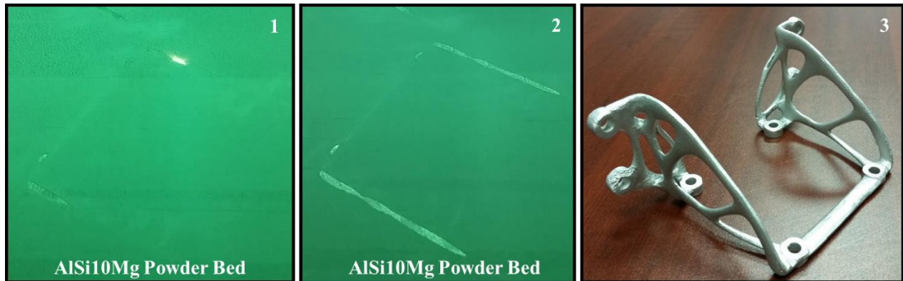
Figure 4.33: Images (1) through (2) depict the DMLS process used to create the final (3) AMM part [17]
