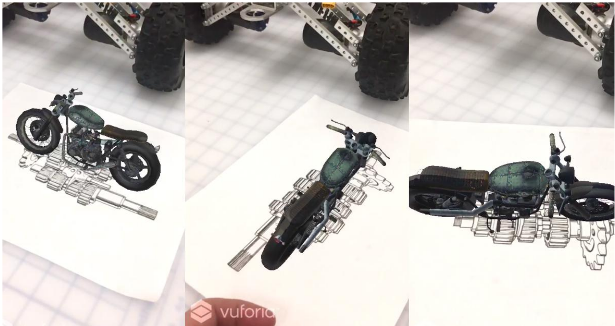
Figure 25: Demonstration of Vuforia's trigger technology, 2D image spawns 3D unity model
