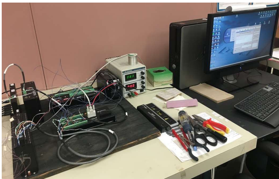
Figure C6. Campbell Scientific digital system and DC power supply connected to the PC via 8 conductor cable from datalogger (CR-1000).
