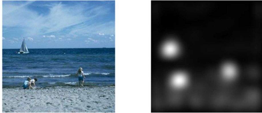
Figure 2.23 Example of cognitive saliency prediction results. Image (Left) and saliency map for it (Right), Accessed at: [32]
