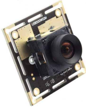
Figure 3.8 ELP OV5640 Sensor (Taken from the manufacturer's online store)
