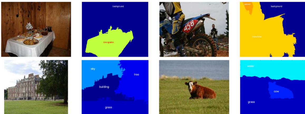
Figure 2.21 Example of semantic segmentation results, Accessed at: [27]
