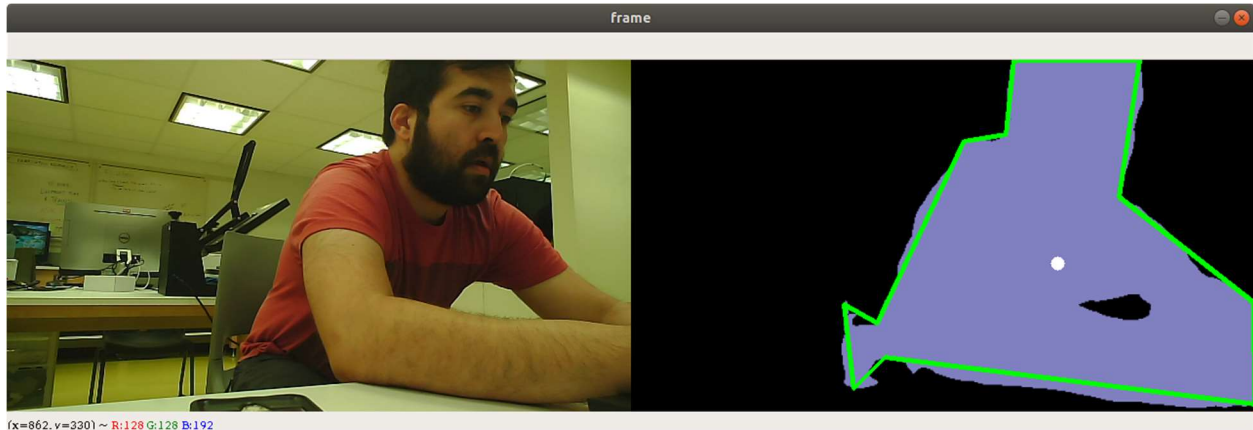
Figure 3.62 (Left) incoming frame (Right) DeepLab output + segmentation outline + Moments
