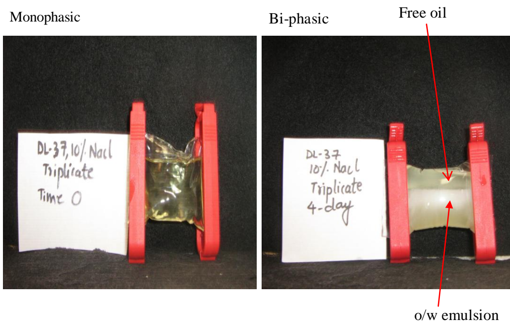
Figure 5.4: Microemulsion images before (A) and after (B) release. Image (A) is the initial, optically-clear w/o microemulsion and (B) is the phase-separated o/w emulsion (with excess oil) after day 4 of release.
