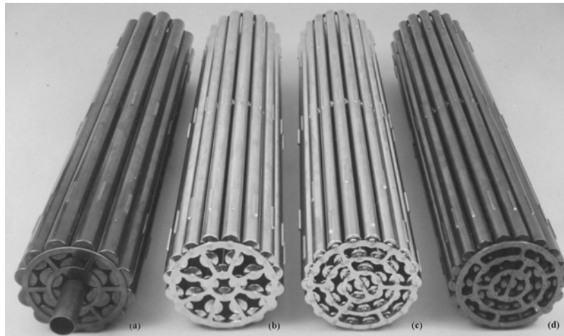
Figure 1.4 Four fuel bundle designs: (a) Gentilly-1 bundle; (b) Pickering 28-element bundle; (c) Bruce 37-element bundle; (d) Gentilly-2 prototype bundle. (Courtesy to CANTEACH at http://canteach.candu.org )
