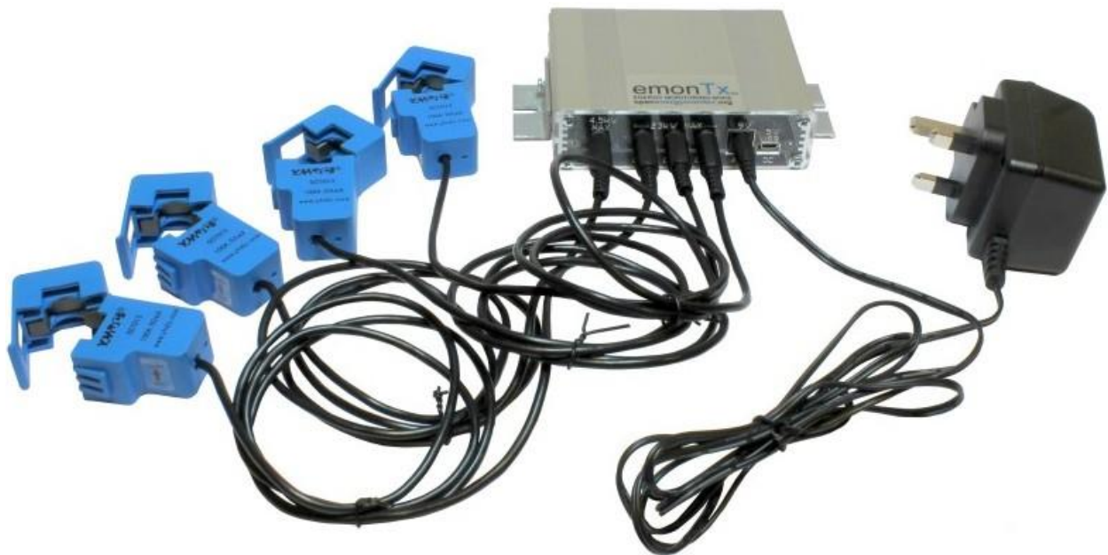
Figure 3-2: emonTx V3 ruggedized power and temperature sensing now Imaged adapted from http://openenergymonitor.org/emon/modules/emonTxV3
