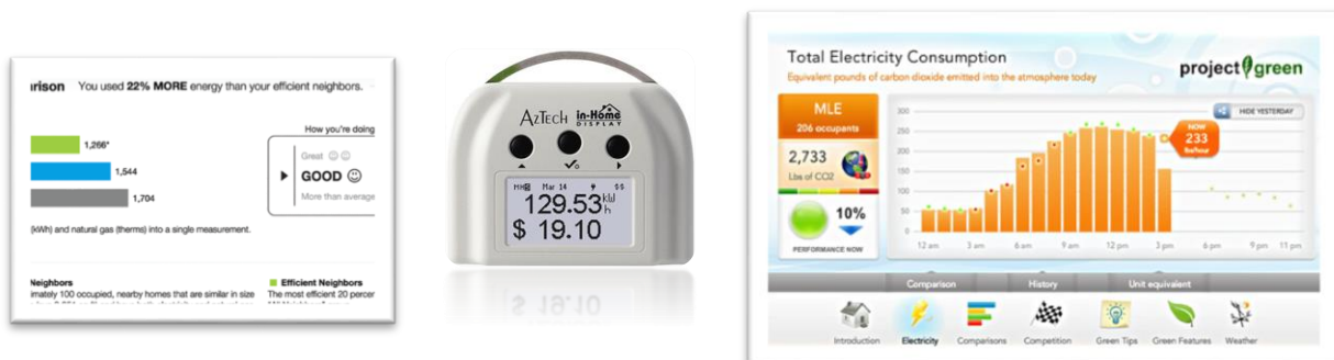
Figure 1-1: Examples of different feedback approaches (From left to right). OPOWER paper bill shows neighborhood comparisons. Aztech In-Home Display shows aggregate home energy consumption. LucidDesign Building Dashboard is a web-based portal offering interactive views of energy use.
