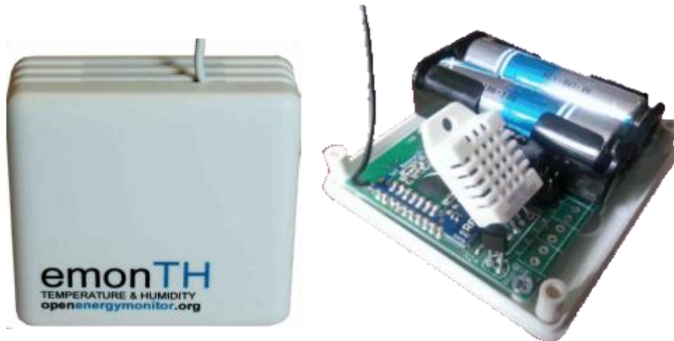
Figure 3-3: emonTH temperature and humidity, battery-powered sensing node Imaged adapted from http://openenergymonitor.org/emon/modules/emonTH
