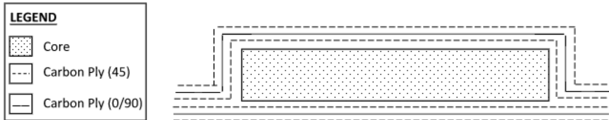
Figure 48: Ply Orientation, Stack-up Sequence and Number of Plies for the NLG Bay Door
