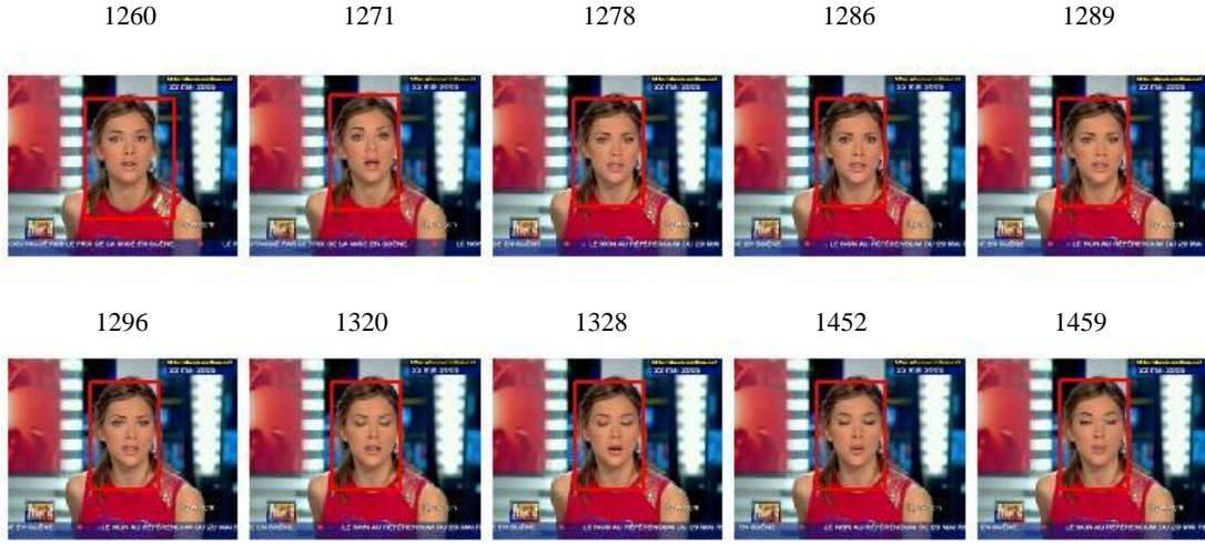
Figure 4.6 Sample sequences from the test videos under good illumination condition, trained face detector with local normalization are applied on each frame. The frame numbers are marked above.
