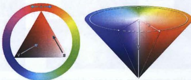
Figure 4.17: An HSV color wheel (left) allows the user to quickly select a multitude of colors. The conical representation (right) of the HSV model is well-suited to visualizing the entire HSV color space as a single object. Notice that the triangle in the left image corresponds to one face of the cone cross section in the right image [48].
