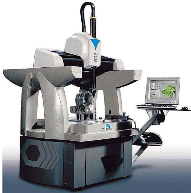
Figure 2-3: Modern CMM Machine [32]
