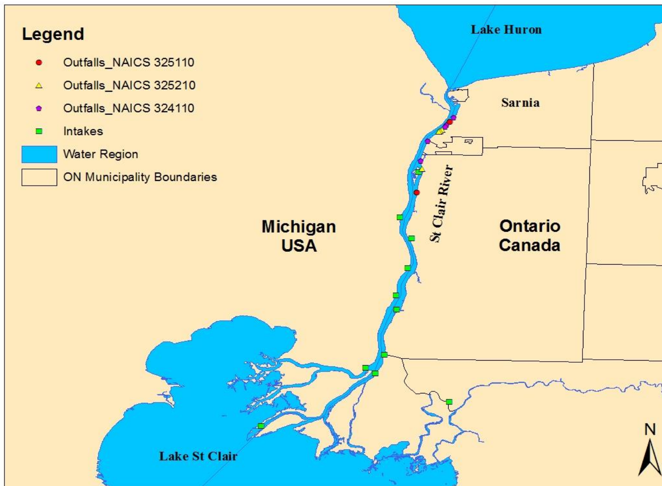
Fig. 3.10: Spatial characteristics of benzene spills by NAICS codes and the water treatment plant intakes along the St. Clair River.
