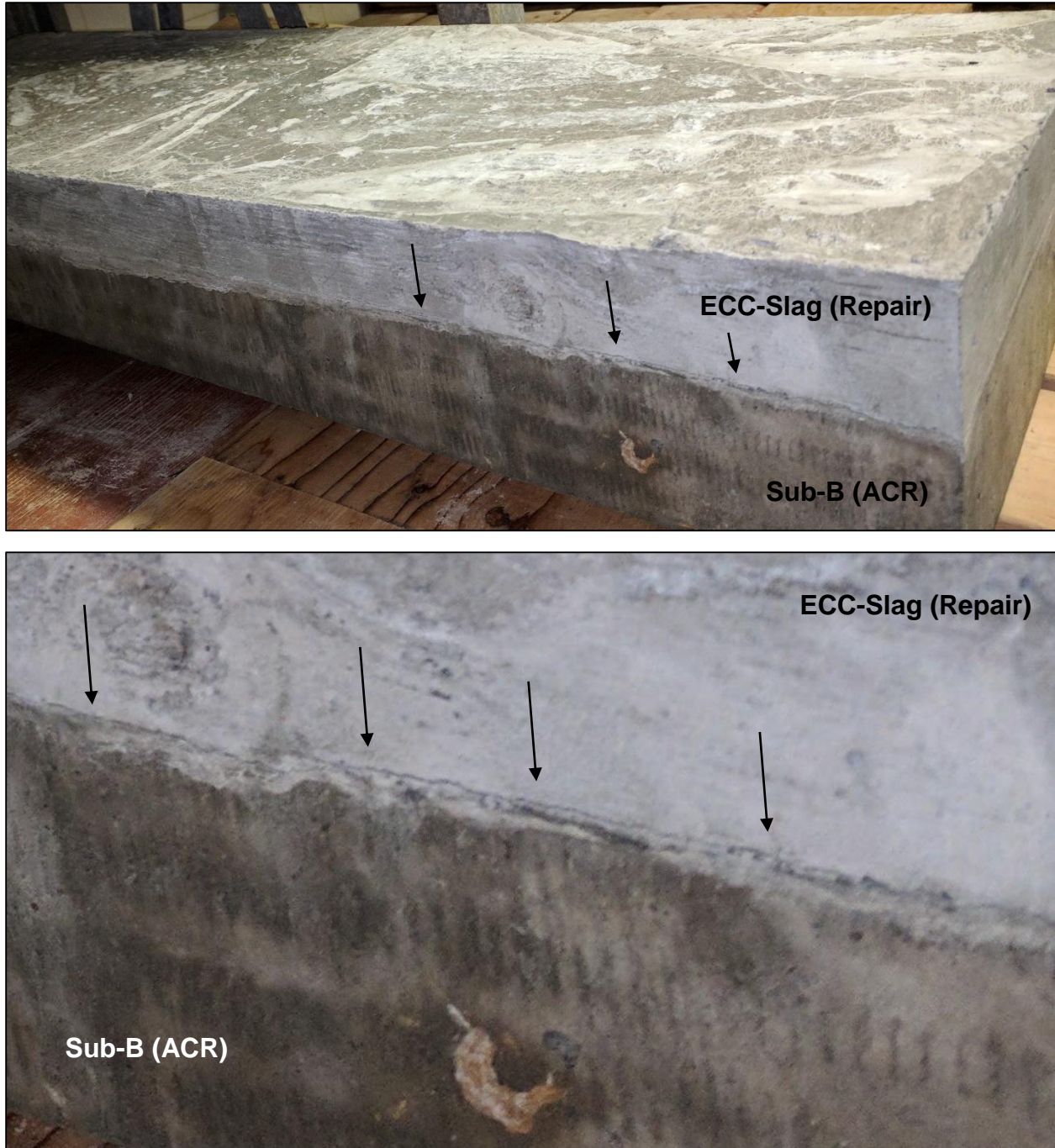
Figure 4-28: Start of Debonding Crack for the ECC-Slag at 1M-Curing
