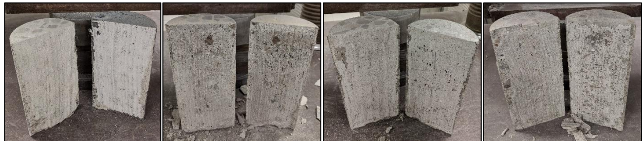
Figure 3-26: Typical Splitting Failure-Smooth Surface (UHPC, ECC, SCC, & NC)
