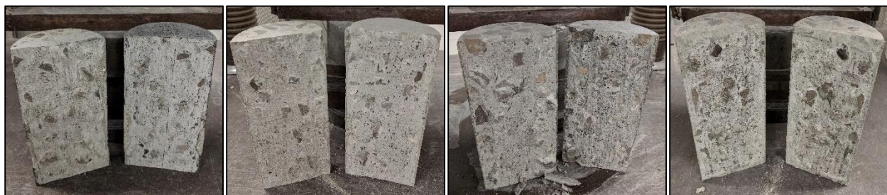
Figure 3-27: Typical Splitting Failure-Rough Surface (UHPC, ECC, SCC, & NC)
