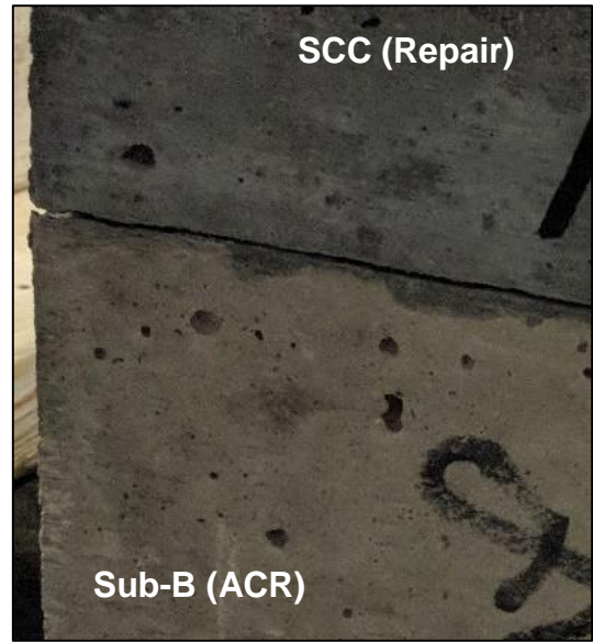
Figure 4-31: Debonding Crack for the SCC at 2M-Curing + 5M
