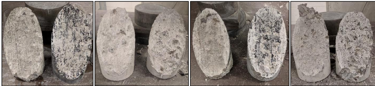
Figure 3-24: Typical Slant Shear Failure-Rough Surface (UHPC, ECC, SCC, & NC)
