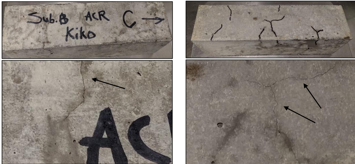
Figure 4-26: Expansion Cracks on the Sub-B Prisms During 2M-Curing + 5M
