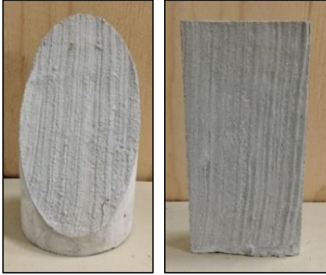
Figure 3-7: Typical Smooth Surface Texture
