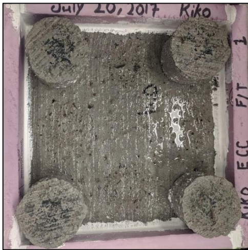
Figure 4-21: ECC-Slag Pull-off Slab with 4 Specimens at 5C-F&T (Debonded)
