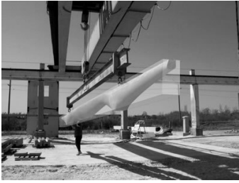
Figure 18: A fabric formed concrete beam by Mark West at the University of Manitoba.
