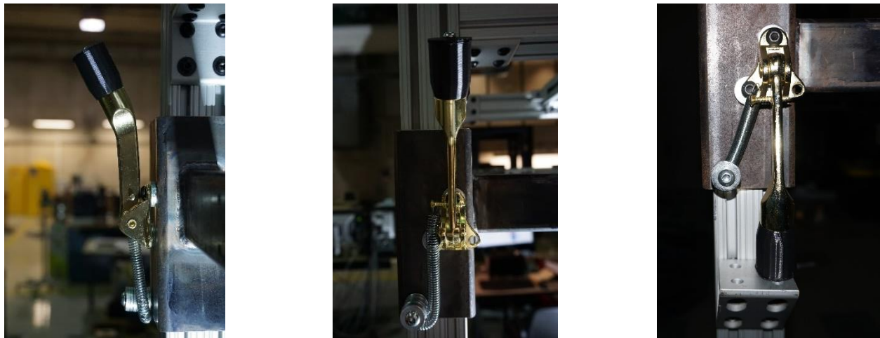
Figure 23 – Spring loaded impactor stop (a) side (b) front pre-impact position (c) front post-impact position
