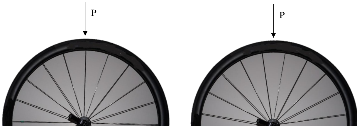
Figure 25 – Loading locations for impact test
