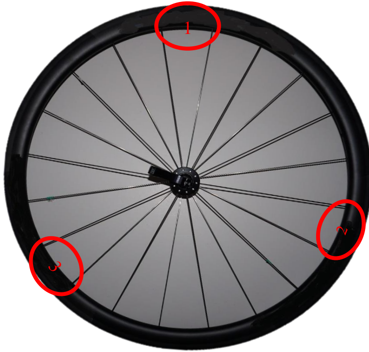
Figure 28 – Impact locations on wheel under test
